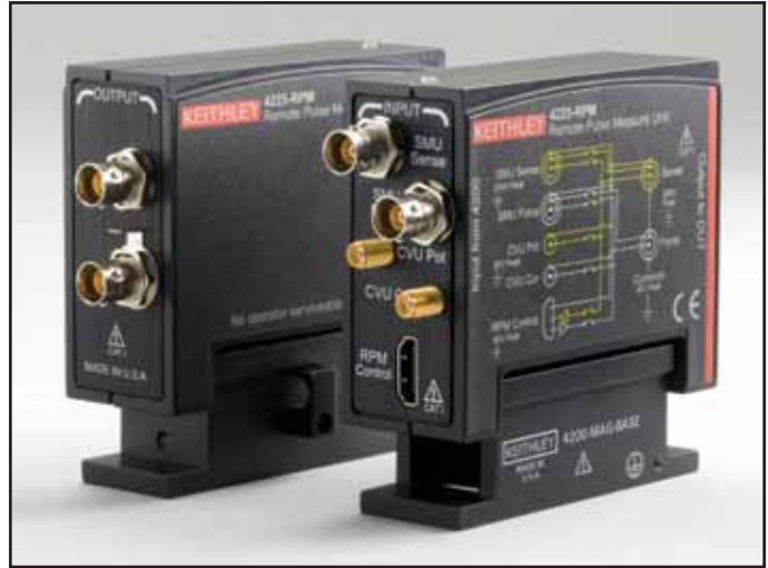
The Model 4225-RPM Remote Amplifier/Switch can be mounted close to the probe needles to reduce the cable effects when performing pulse or other ultra-fast I-V measurements.
