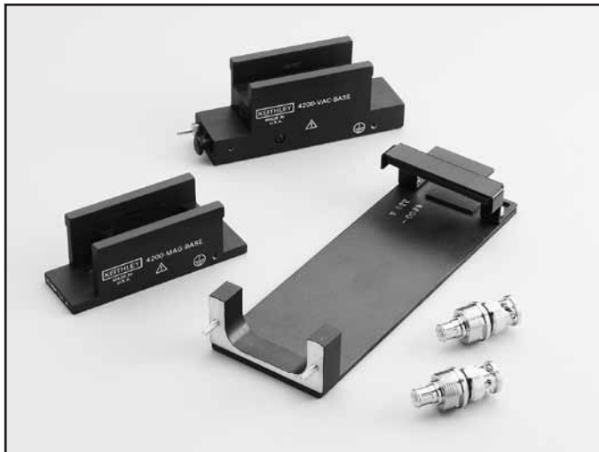
An optional vacuum (Model 4200-VAC-BASE) or magnetic (Model 4200-MAG-BASE) platen mounting base allows the PreAmp to be located next to manipulators on the chuck platen, eliminating measurement problems caused by long cable lengths when performing ultra-low current measurements.
