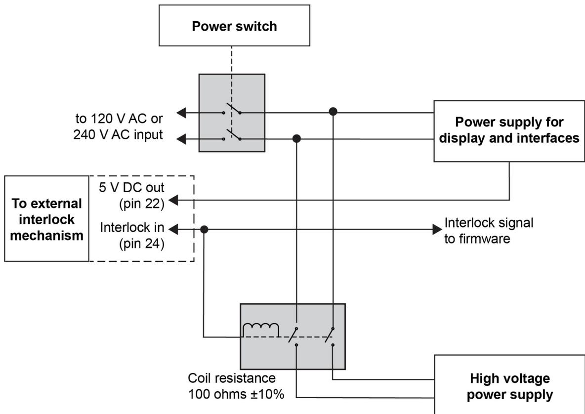
The output of the Model 2657A can only be turned on when the interlock is engaged. Attempting to turn on the output when the interlock is disengaged will generate error code 802, "Output Blocked by Interlock."
