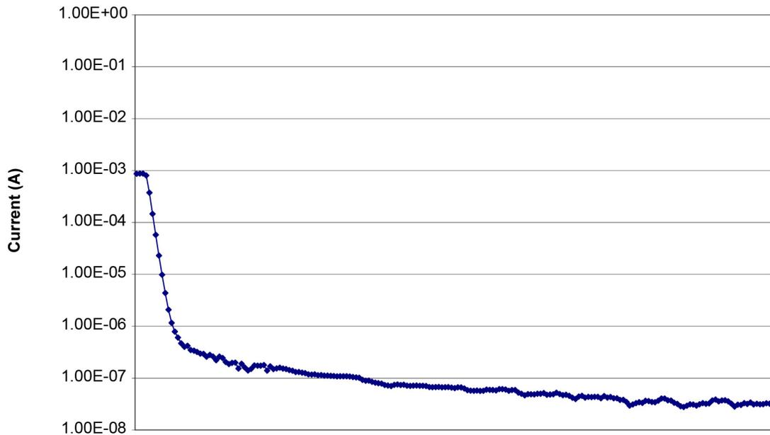
**Figure 33: Sample data for capacitor leakage test**
