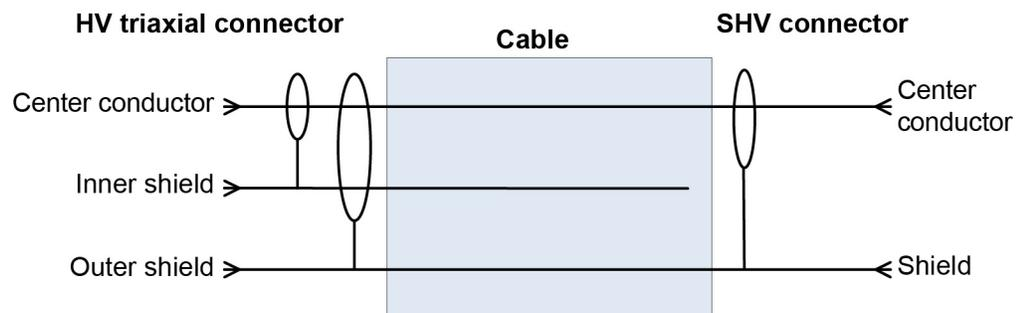
Be aware that when you connect the Model SHV-CA-553 cable assembly to the SLO/LO triaxial connector on the rear panel of the Model 2657A, the LO terminal is the inner (or first) shield. Therefore, the LO terminal is not carried to the SHV end of the Model SHV-CA-553 cable assembly. Use the LO triaxial connector on the rear panel of the Model 2657A to access Output LO.
