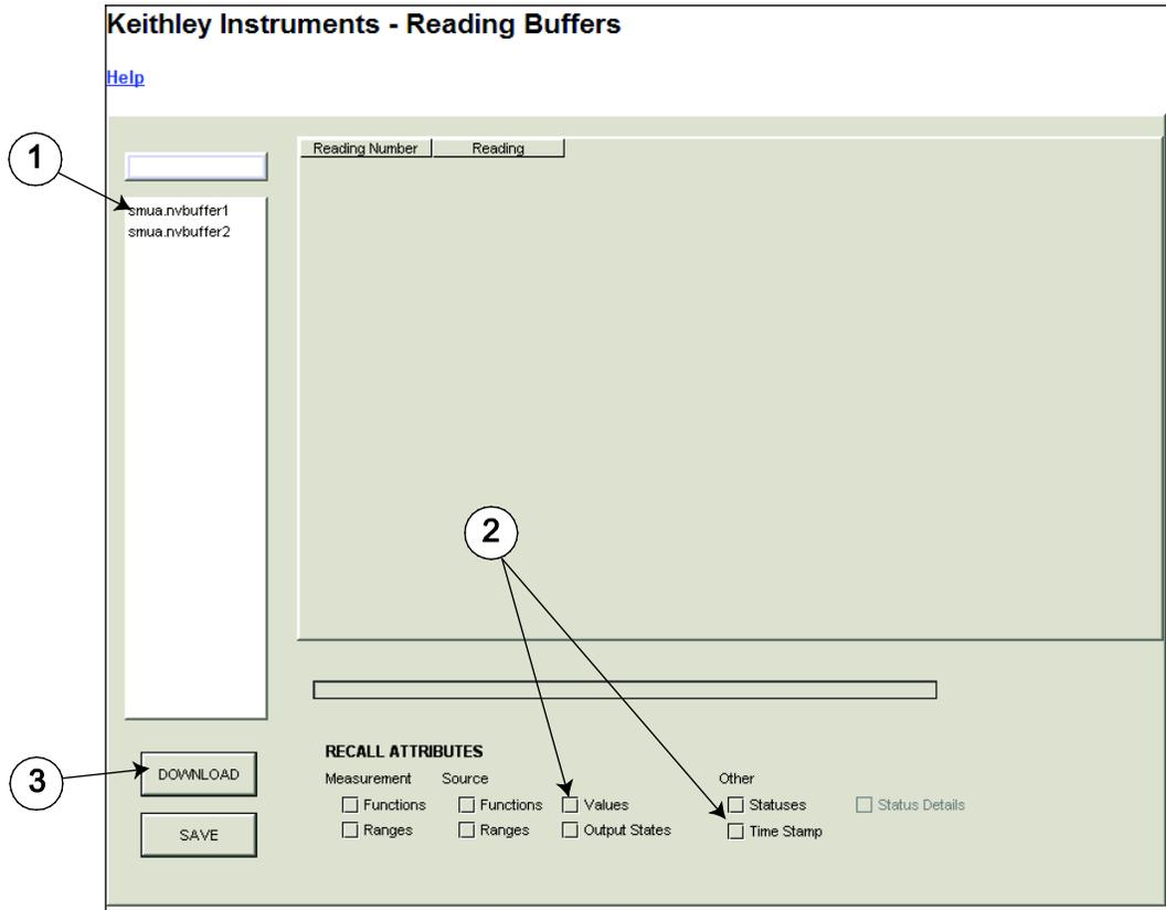
5. The table displays the present buffer data. Notice that the Source Value column is not populated. To collect source values, before taking readings, use TSB Embedded to set the following attribute: `smua.nvbuffer1.collectsourcevalues = 1`.
