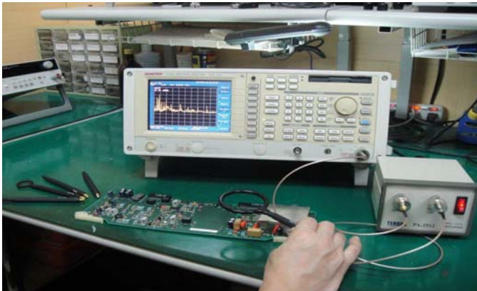
Loop Probes offer varying sensitivities to H-Field emissions.
